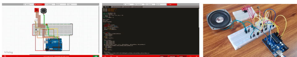
Fig. 5. User-study task. Left: The circuit plan; Middle: The code; Right: The completed physical circuit.
